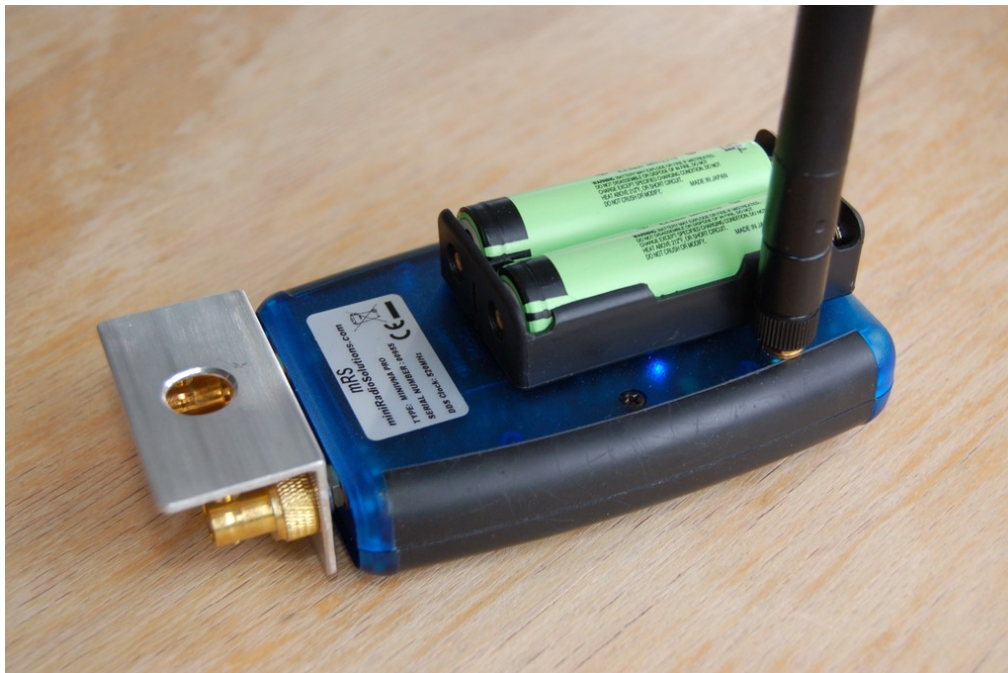
Figure 1: External view of the heavily modified miniVNA PRO showing the external Li-ion battery pack, an external 2.4 GHz Bluetooth antenna and an aluminium hanging bracket held down by two SMA to BNC connector adapters. A steady blue LED is indicative of a stable Bluetooth connection.
