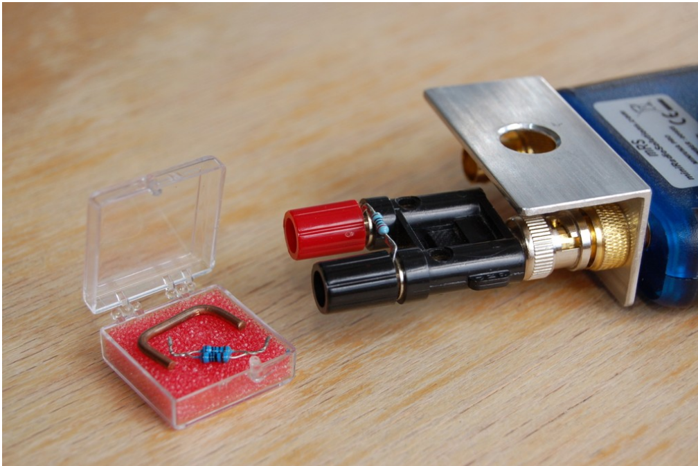
Figure 6: A calibration kit for banana terminals. The tiny plastic box on the left contains a short and a 50\ \Omega load consisting of two high-precision 100\ \Omega low-inductance metal film resistors in parallel. On the right, a high-precision 200\ \Omega low-inductance metal film resistor for measuring components of CL-OCFD antennas .
