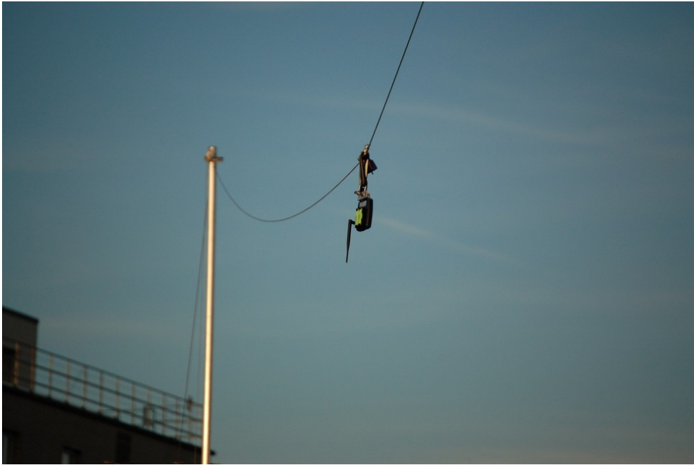
Figure 4: The modified miniVNA PRO hanging from the center of a HF dipole at about 15 m (50 ft) above ground. A balun is not required for taking accurate measurements. The VNA can be read from the comfort of my home even though there are quite some 2,4 GHz WLAN signals present in this urban environment. The two 3350 mAh Panasonic NCR18650B Li-ion cells in parallel provide more than enough «juice» for a whole day of measurements.
