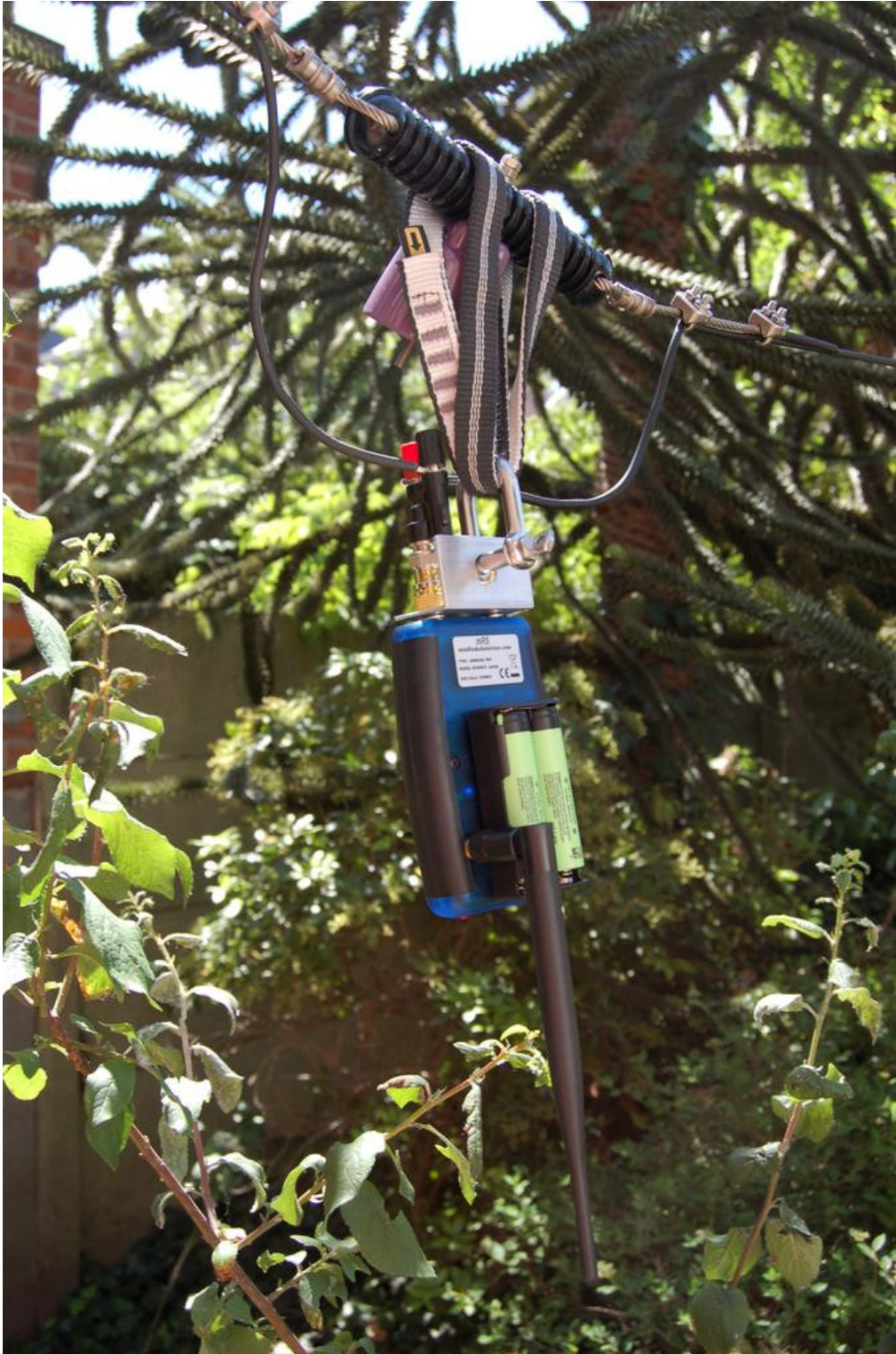
Figure 5: Detail of the modified miniVNA PRO hanging from a lowered wire antenna in my urban jungle. A stainless steel D-shackle and a 30 cm (1 ft) mountaineering sling are used to secure the VNA to the antenna's center insulator. Prior to taking any measurements, the VNA was properly calibrated at the banana terminals.
