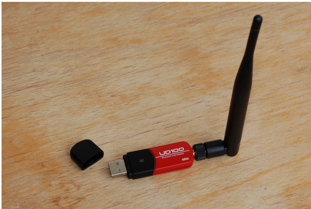
Figure 3: The Sena Parani-UD100 Class 1 (100 mW) Bluetooth 4.0 dongle connected at its RP-SMA port to an aftermarket 2,4 GHz dipole antenna provides an open field signal at a range of up to 600 m.
