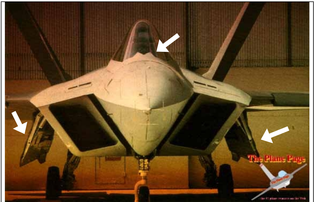
Figure 1.11: Indented surface discontinuities on the F-22's fuselage
