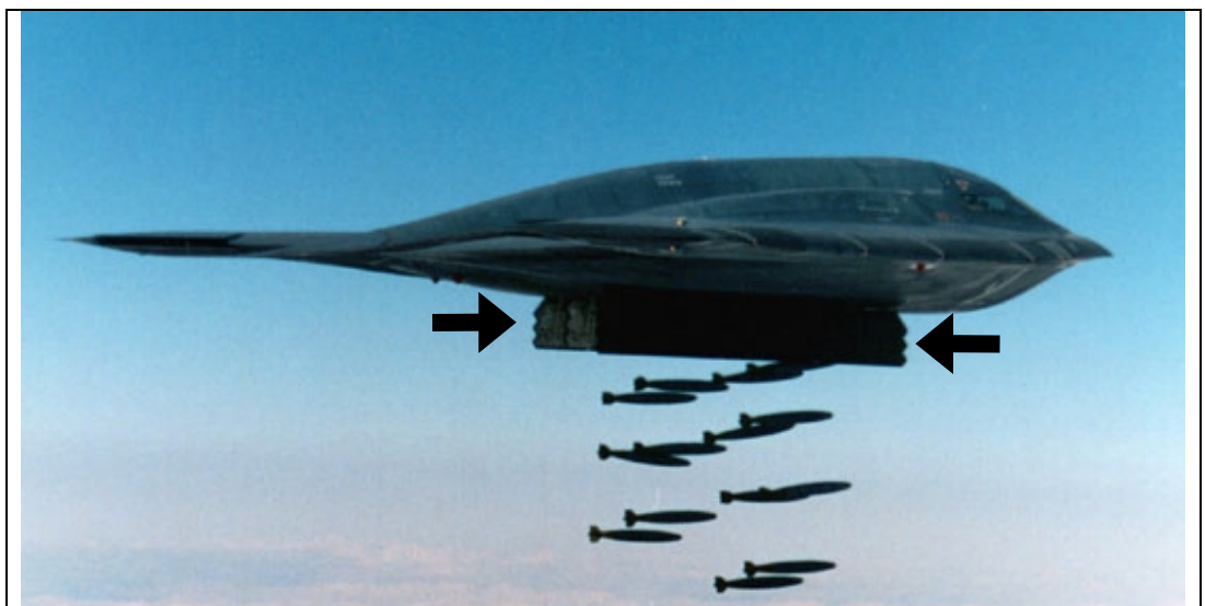
Figure 1.9: The indented payload doors of a B-2
