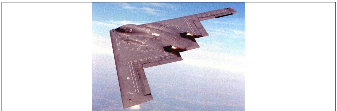
Figure 1.8: The B-2 stealth bomber plane. A flying-wing design and an indented rear edge result in an extremely low RCS value.
