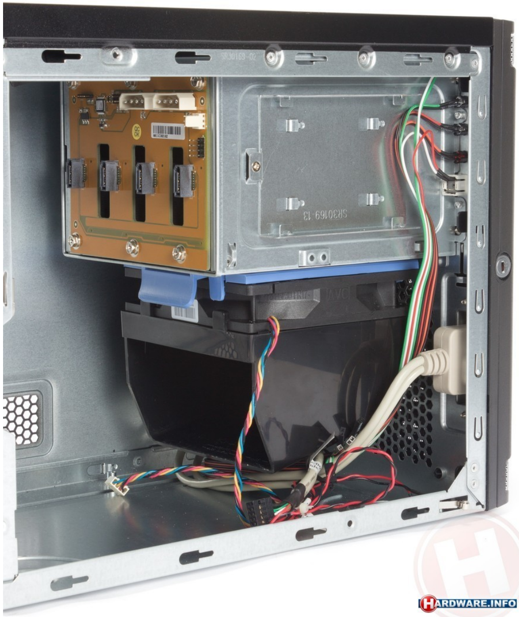
Figure 9: Chenbro SR30169 SATA connections
