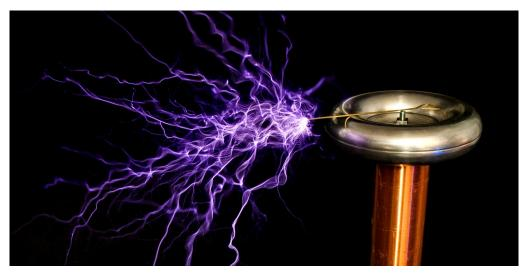
Figure 5: Voltage breakdown of the air at one end of a Tesla coil. *Source:* oneTesla
