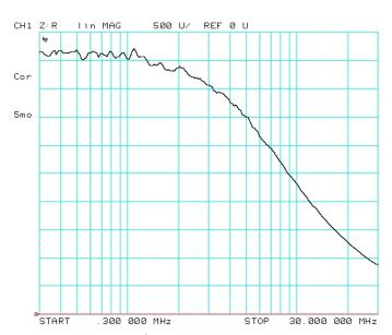
impedance, with each graticule line 500 ohms. Two inches of typical 50 ohm coaxial cable represents 5.3pF shunt capacitance, with an impedance of 1000 ohms at 30 MHz.
