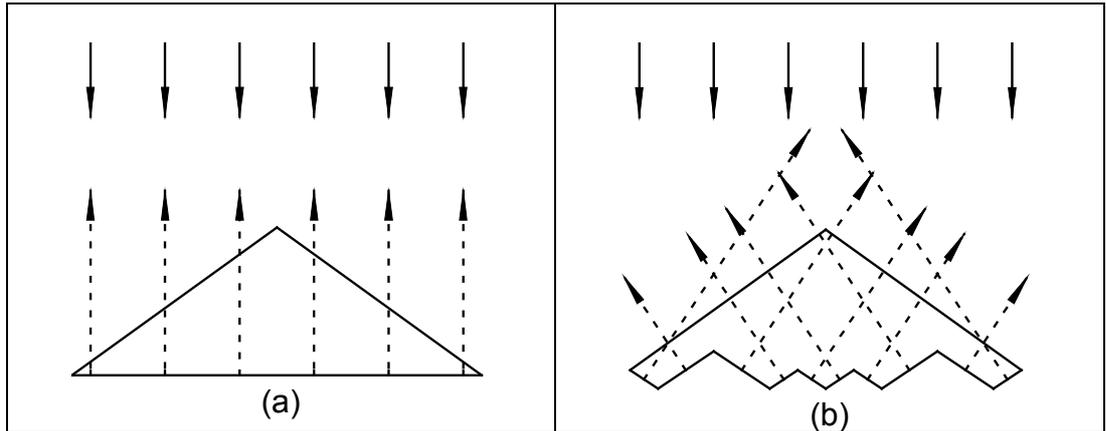
Figure 1.7a: Edge diffraction from the trailing edge of a straight wing
