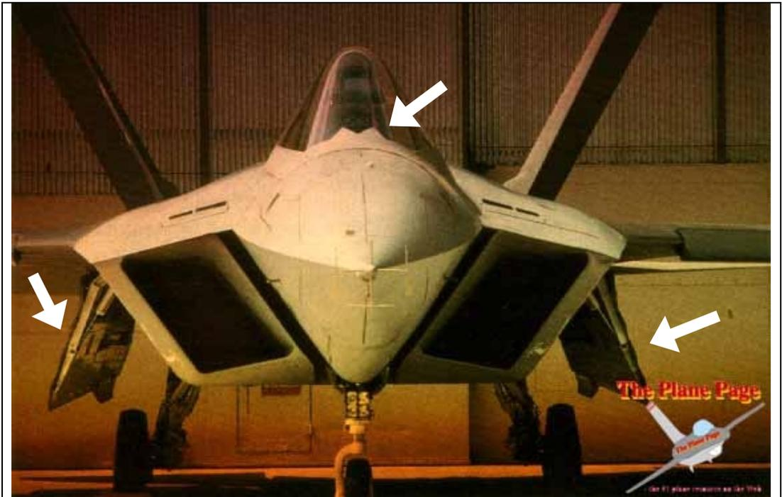
Figure 1.11: Indented surface discontinuities on the F-22's fuselage
